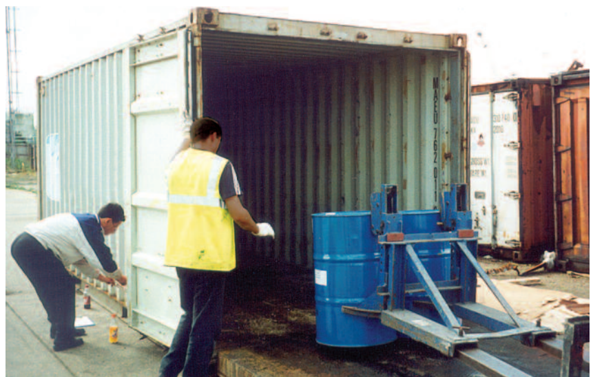
Drums being packed with drum clamps
