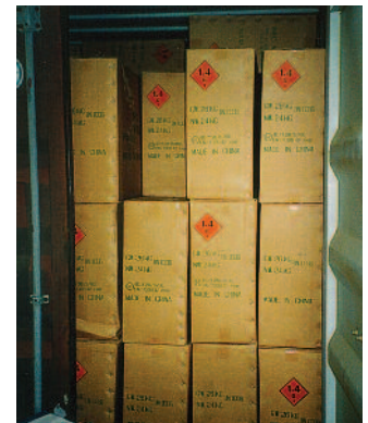
Packages stacked with dangerous goods labels facing the door
